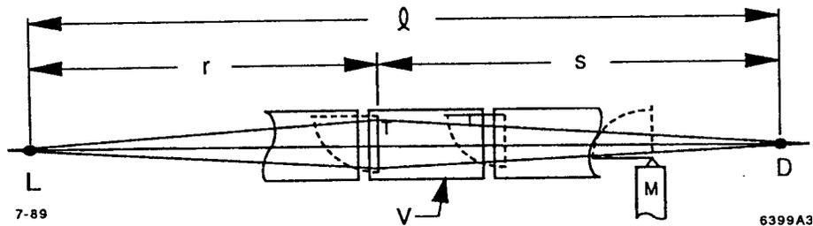
Fig. 1. Schematic illustration of the SLAC alignment system. *T* is one of 294 rectangular Fresnel lenses which focus laser light *L* to an image at the detector *D*. *V* is one of 60-cm diam. vacuum pipes, each 12 meters long which also serve to support the accelerator
