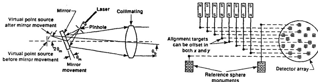
Fig. 2. Schematic of the Poisson Alignment Reference System
