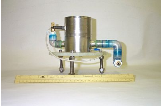
Figure 1: Budker HLS sensor
